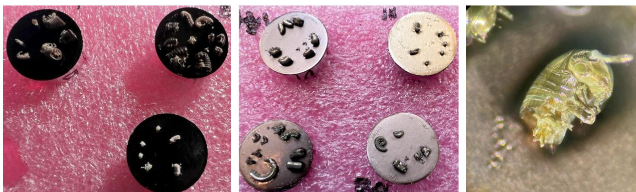
Figure 1: Specimens glued to aluminium stubs and coated with gold.
