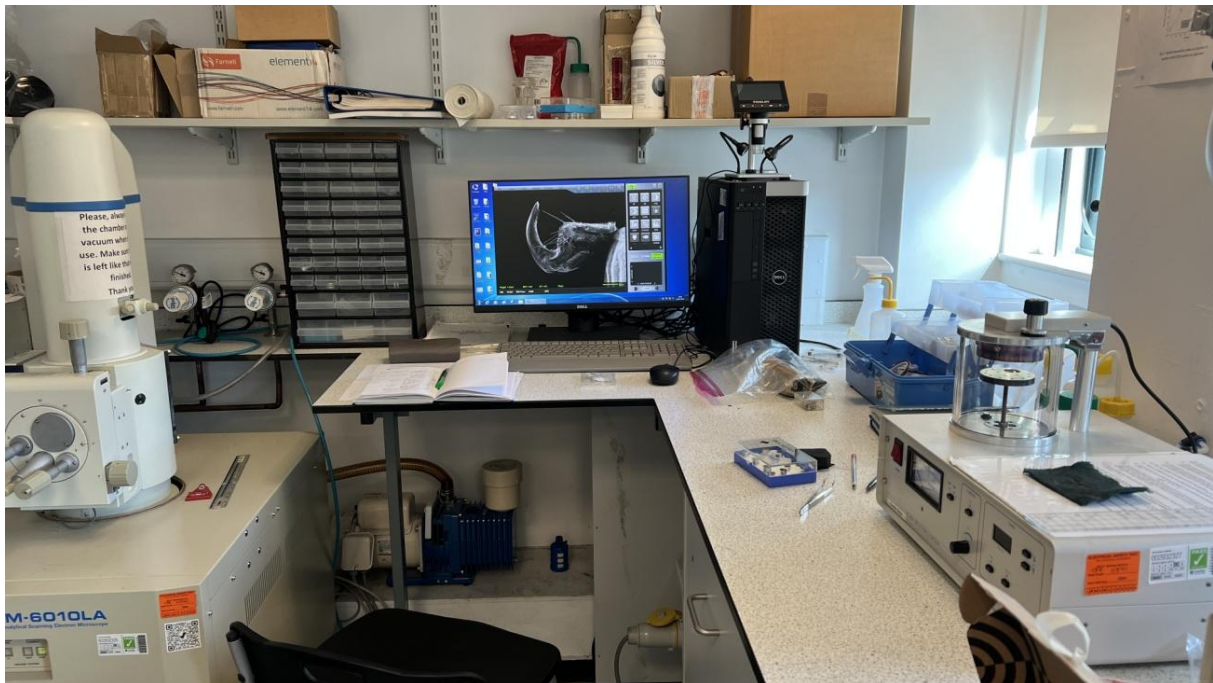
Figure 2 : The JEOL JSM-6010LA Scanning Electron Microscope (left), user interface and gold sputter-coater (right)
